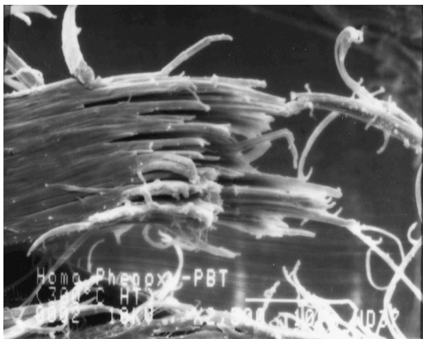
Figure 6 Fibrillar morphology of PPBT fibre after heat treatment at 300°C
